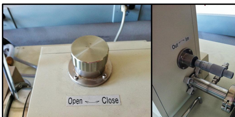
Figure 6. Control knobs for the nickel electrodes, left, and the sample probe, right.
